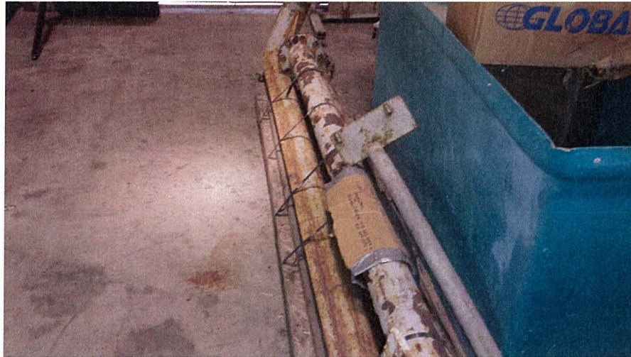
Stored Metal Pipes with Deteriorating Paint.
